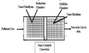
Figure 4. Three way catalytic convertor
