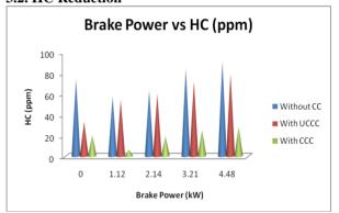
Figure 8. HC Reduction based on Brake Power
