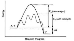
Figure 3. General Diagram of Potential Energy
