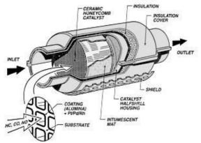
Figure 5. Three way catalytic convertor
