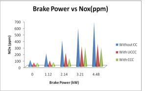
Figure 7. NOx Reduction based on Brake Power
