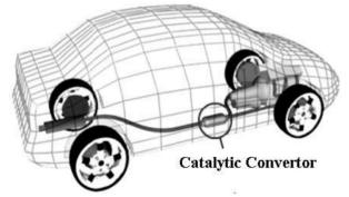
Figure 2. Placement of Catalytic Convertor
